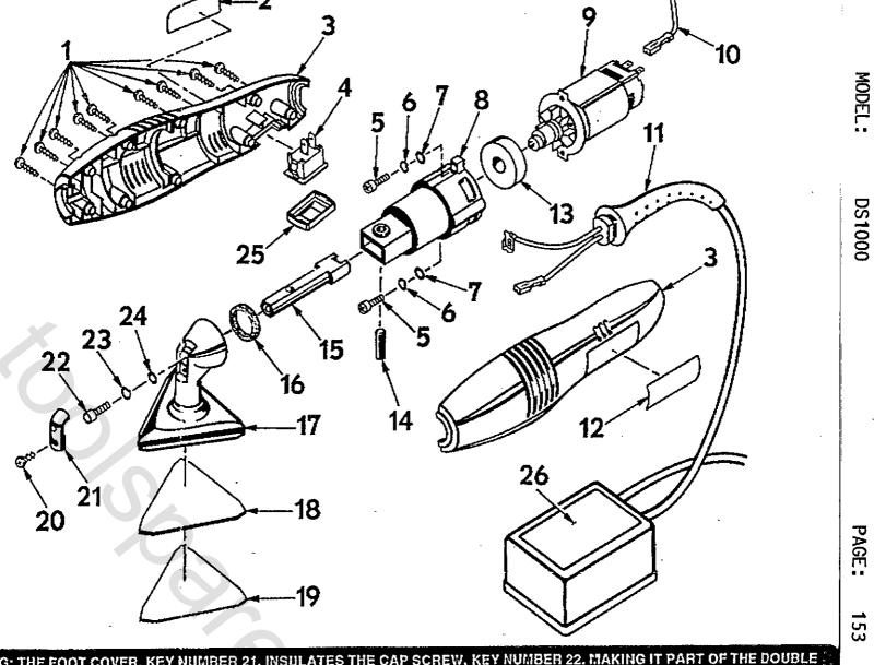
WARNING: THE FOOT COVER. KEY NUMBER 21. INSULATES THE CAP SCREW, KEY NUMBER 22. MAKING IT PART OF THE DOUBLE INSULATED SYSTEM. THEREFORE, IT MUST ALWAYS BE REPLACED WHEN REPLACING PARTS OR MAKING REPAIRS TO THIS TOOL.
