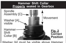
Washer [A] must be visible above Hammer Collar [B] on Spindle Assembly [C]
